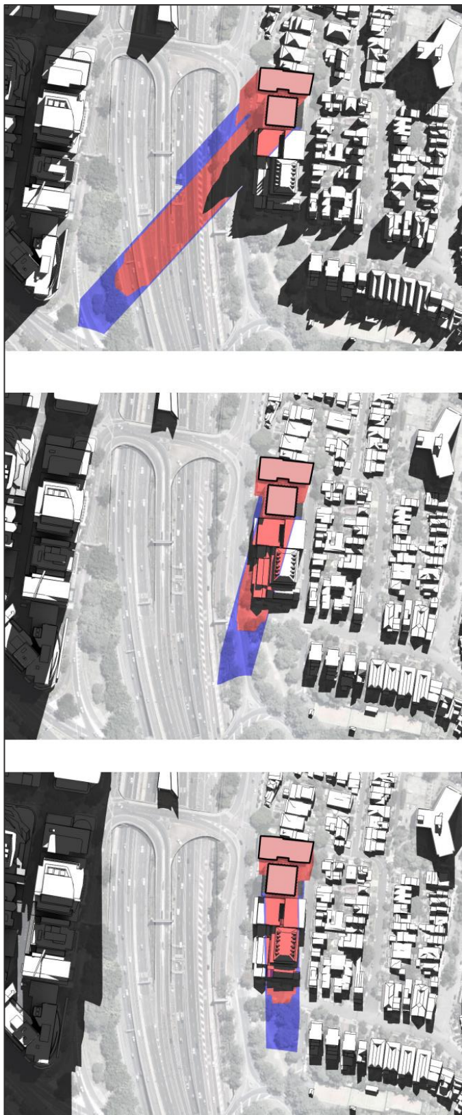
Figure 14. Concept scheme shadow diagrams on 21 June at 9am (top), 11am (middle) and 12pm (bottom) red shadow represents existing building blue shadow represents proposed building (source: Grimshaw Architects - urban design package )
